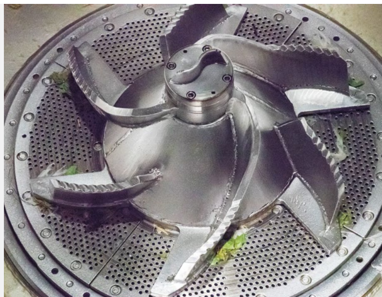
Innovative new pulper rotor geometry increases disintegration efficiency and shortens retention time. This in turn lowers energy consumption and increases pulping capacity.
