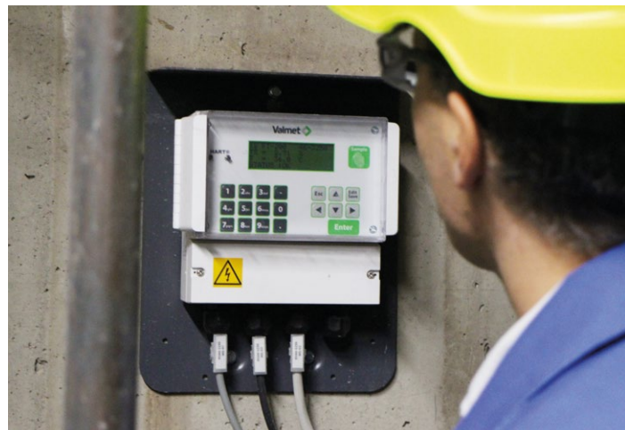
Valmet TS is a third-generation microwave solids transmitter, designed for use in the demanding pulp and paper mill environment. It uses patented microwave-based technology to measure total solids content, and is unaffected by flow rate or the color of the process stream.
